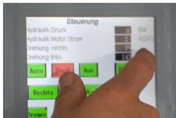
Another great operational feature is the ability to switch between automatic and manual control of the wind turbine, safety devices (e.g. brake) and distribution/storage of generated power.
